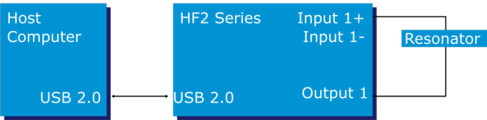
Figure 4.27: PID connection with HF2 instrument
